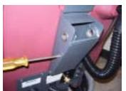
Use philips screwdriver to unscrew 4 screws and remove cover.
